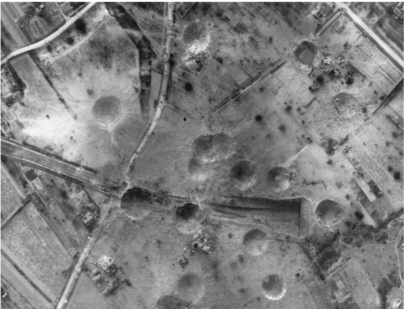
Post strike imagery of the 617SQN attack on the Saumur Railway Tunnel and Bridge clearly showing the large craters caused by the 617SQN Tallboy bombs along the rail cratering the rail line and just after the entrance to the tunnel. (IWM)
